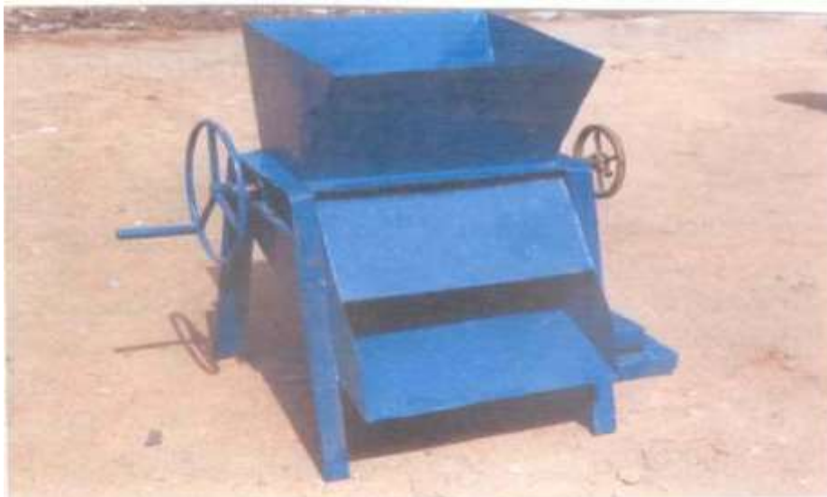
Plate 5. A Dual - Operational Cassava Grating Machine, Source: (Ndaliman , 2006)
