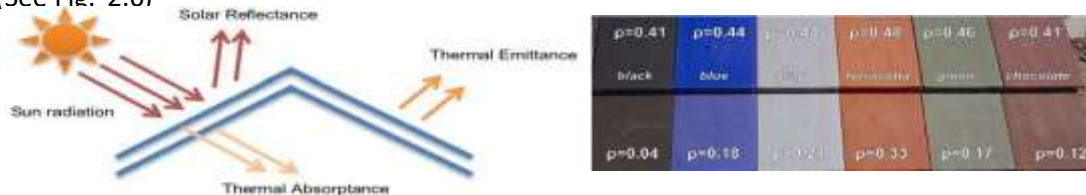
Figure 2.6. Showing Cool roof mechanism and Cool dark colour roofs Source: American roof tile coatings (2020)
