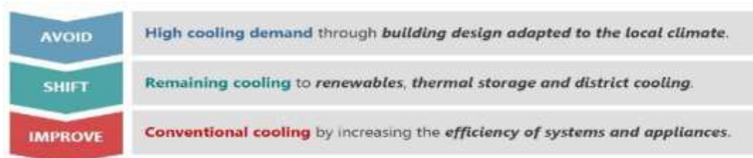
Figure 2.1. Steps for low carbon buildings
