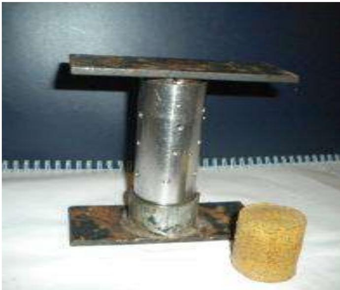
**Figure 1: The constructed Briquette mould (Length=15 cm ID=30 cm, OD= 35 cm)**
