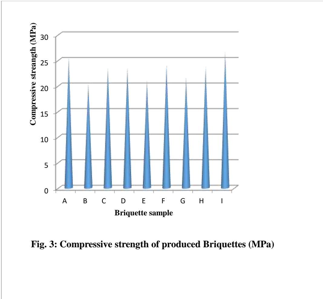
**Fig. 3: Compressive strength of produced Briquettes (MPa)**
